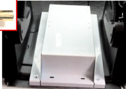
Set the aluminum base into position between the seats, and thread the four hex bolts & washers down through the aluminum base and into the plus-nuts you had just installed. You should remove the protective film from the aluminum base before fastening down.
