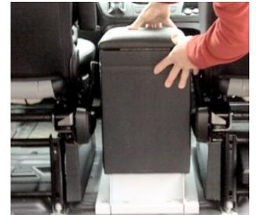
Set the black console onto the aluminum base, making sure that it is centered left-to-right. Also make sure that it's centered such that it overhangs equally on the front as well as the back. Once its set as described, use the four self-drilling screws and fender washers to screw the console down to the aluminum base.
